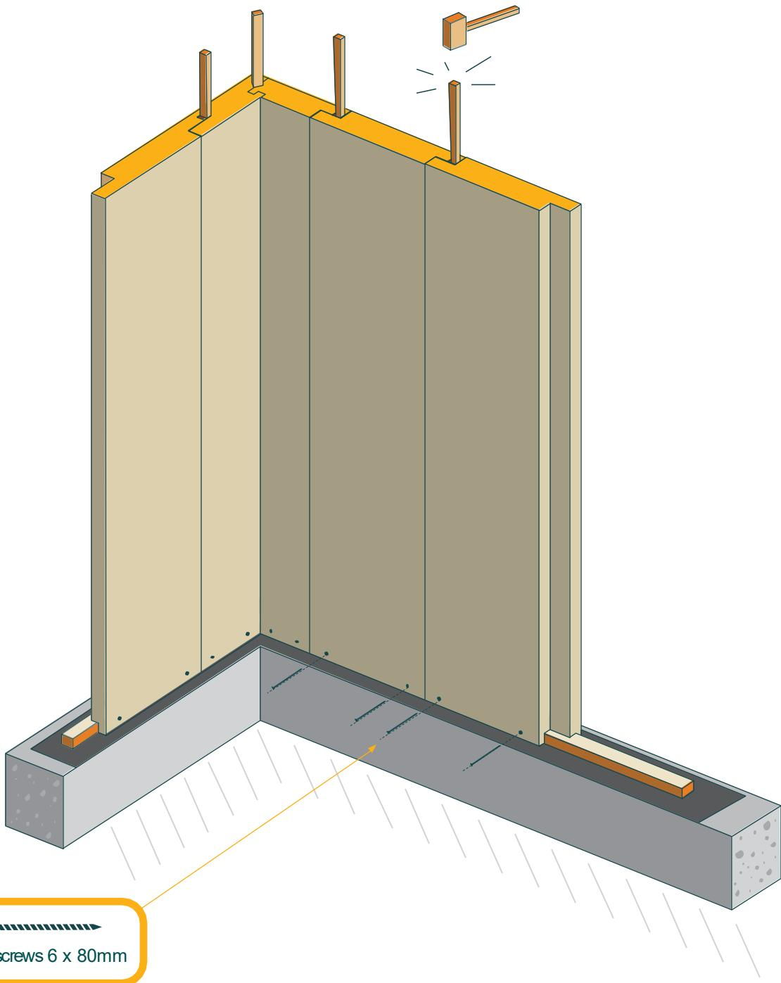
17. When placing KLIK-KLIK wedges, tap the wedges soft way and only partially fix the several panels (soft fix) before you go to Nr.18 (Hard fix)
