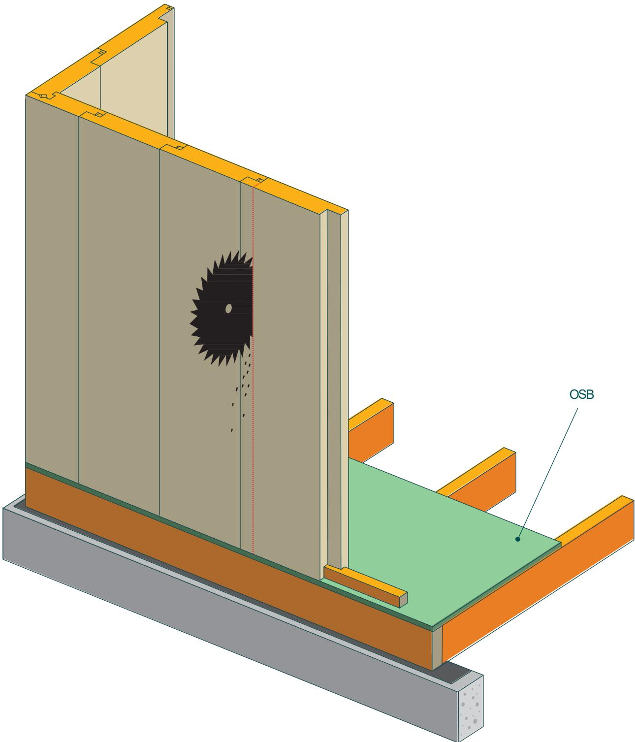
33. In a situation where the panels are mixed up and the wedges are hard fixed (hard fix) and can no longer be removed, we cut the panel so that the wedges can be taken out and the panels can be disassembled. After that, the panel is screwed together with a metal plates and screws
