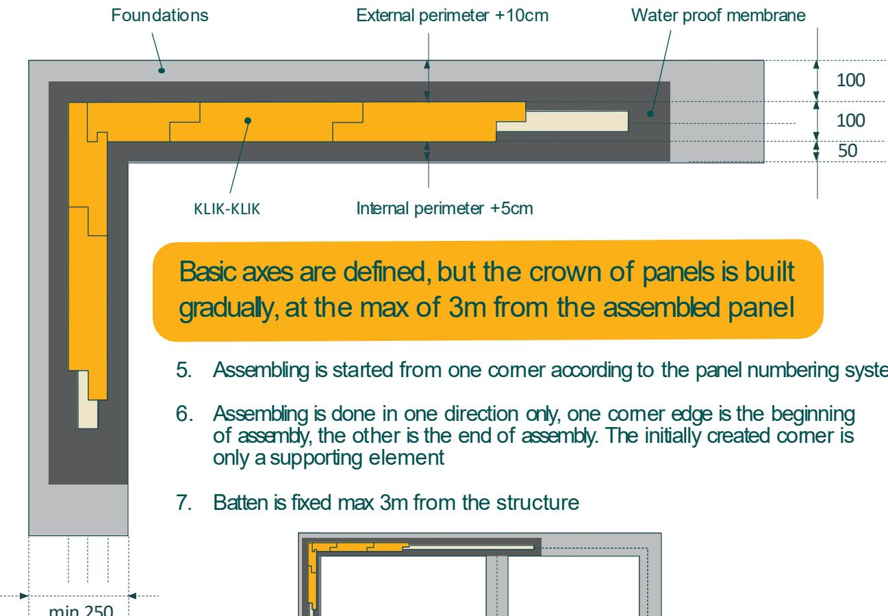
5. Assembling is started from one corner according to the panel numbering system
