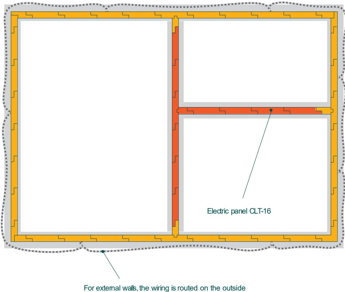
28. Electric panels - CLT-16 - to be used only for internal walls!
