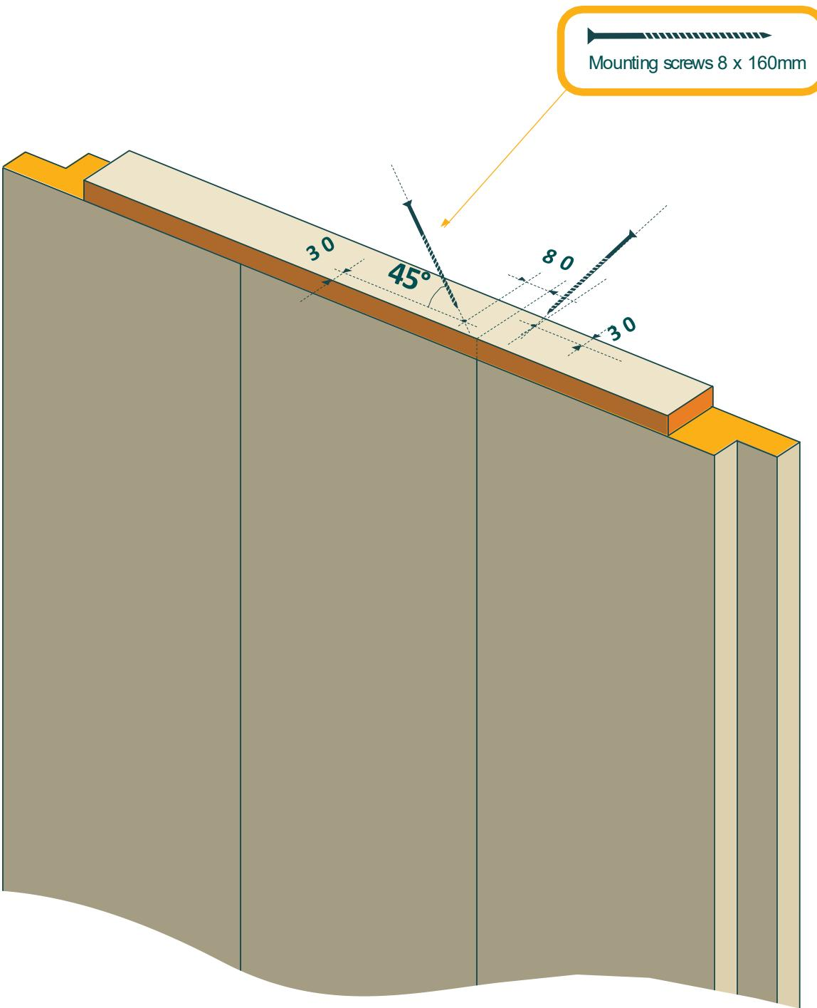
26. Additional screws are used between KLIK-KLIK panels with min dimensions 8x160 mm
