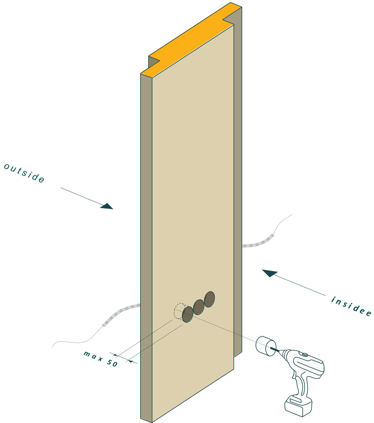
31. For external walls, the electrical wiring is pulled outside and the wires are drilled to the socket from the outside
