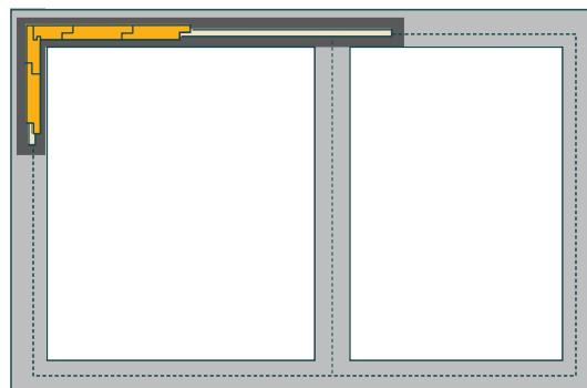
8. The batten is drilled max. 3 m "forward", the drilling is carried out according to pre-set height marks on the axis of the foundation, this is essential if the foundations are not perfectly level
