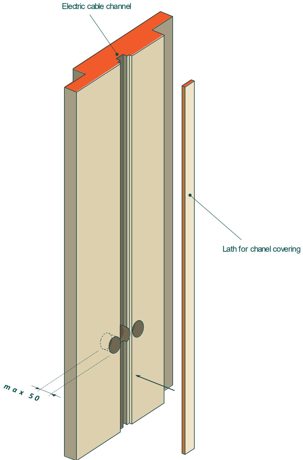
30. A maximum of three rosettes in one panel when installing them on site
