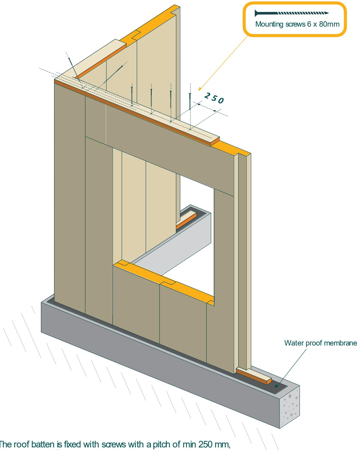
24. The roof batten is fixed with screws with a pitch of min 250 mm, or three screws for one panel
