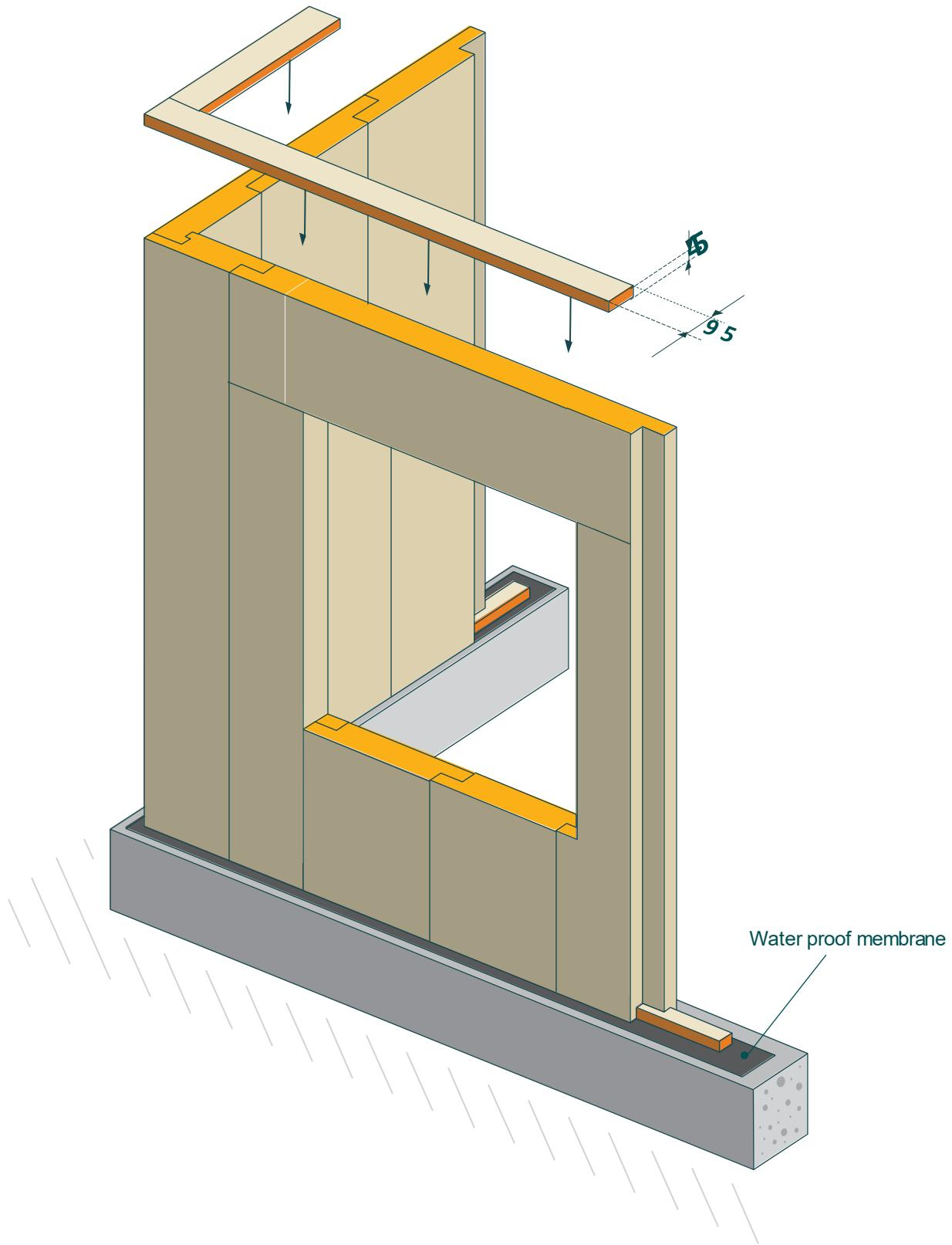
23. Before laying the roof batten, hammer the wedges to the end (hard fix) so that the top plane is smooth
