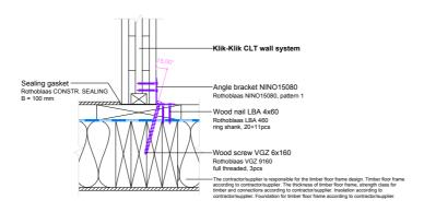
These drawings contain standard solutions designed by KLIK-KLIK for AutoCAD software. ase drawings are intended for architects and structural engineers to use the KLIK-KLIK Wall System...
